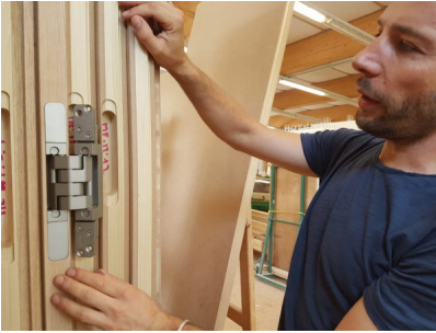
Caption 9: The master carpentry company, Prader, specialises in the production of tailor-made doors. They have been working together with BaSys since 2007, says Hannes Prader. Back then, the partners installed a total of 500 flush-mounted doors with the "Pivota DX 38" concealed hinge in a building complex with 90 apartments. Photo: BaSys
