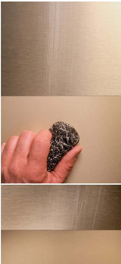
Caption: Lovely to look at, stunning effect: the new, highly scratch-proof matt surface from Homapal is called "Scratch-Resistant Matt", SRM for short, and also comes with anti-fingerprint finish. Photo: Homapal
