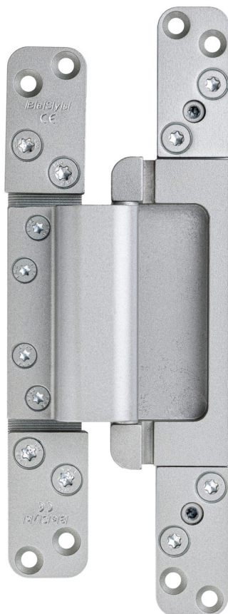
Caption 1: In the old model of the "Masterband FX2 120 3-D FD", the side gap adjustment was still in the leaf of the concealed hinge developed for front doors. When adjusting the side gap, however, the seal in the leaf was sometimes displaced - with negative effects on the tightness which is essential for front doors. Photo: BaSys
