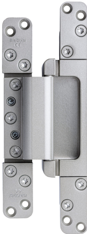
Caption 2: In the new model of the "Masterband FX2 120 3-D FD", all three dimensions of adjustment - the side gap adjustment, the height adjustment and the pressure of the seal - are now located in the frame part of the hinge. The leaf part and the continuous seal enclosed by the hinge remain untouched during adjustment. Photo: BaSys
