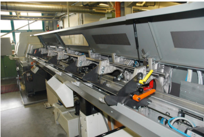
Caption 7: Schwinn plant in Krakow/Poland: Sliding head lathe for bar handles. Photo: Schwinn
