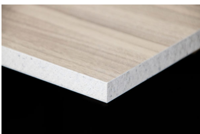
Caption 1: "A2-Solution" is a non-flammable composite element made of a gypsum fibre board and a decorative, 0.7 mm thick laminate coating classified in accordance with DIN EN 438-1 and EN 438-9. Photo: Homapal
