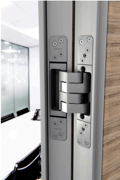
Caption: The concealed hinge "Pivota DX 110 3-D" overcomes claddings of up to 10 mm on both the leaf and frame side. The load capacity is 100 kilograms per pair. Photo: Basys
